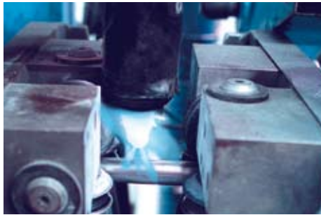
Production: LaserTIG welded aluminium layer
