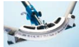
...or using a hydraulic bending machine (for pipes up to 32 mm diameter)
